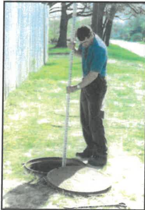
Sediment inspection using a stadia rod
